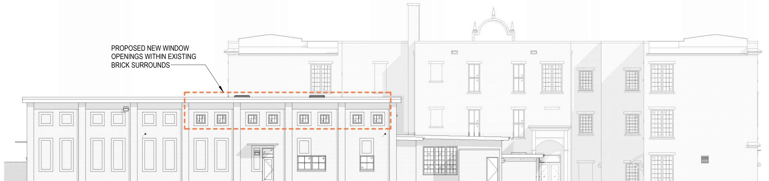
PROPOSED NEW WINDOWS ON WEST / REAR FACADE
