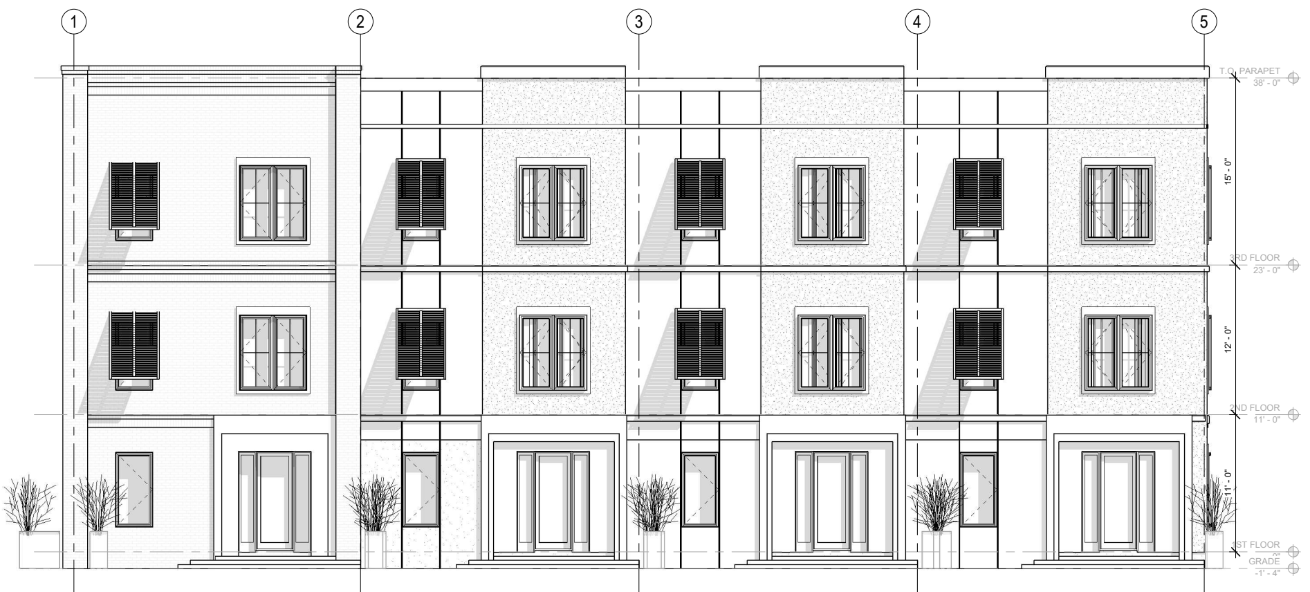
2 BLDG B - EAST ELEVATION SCALE: 3/16" = 1'-0"
