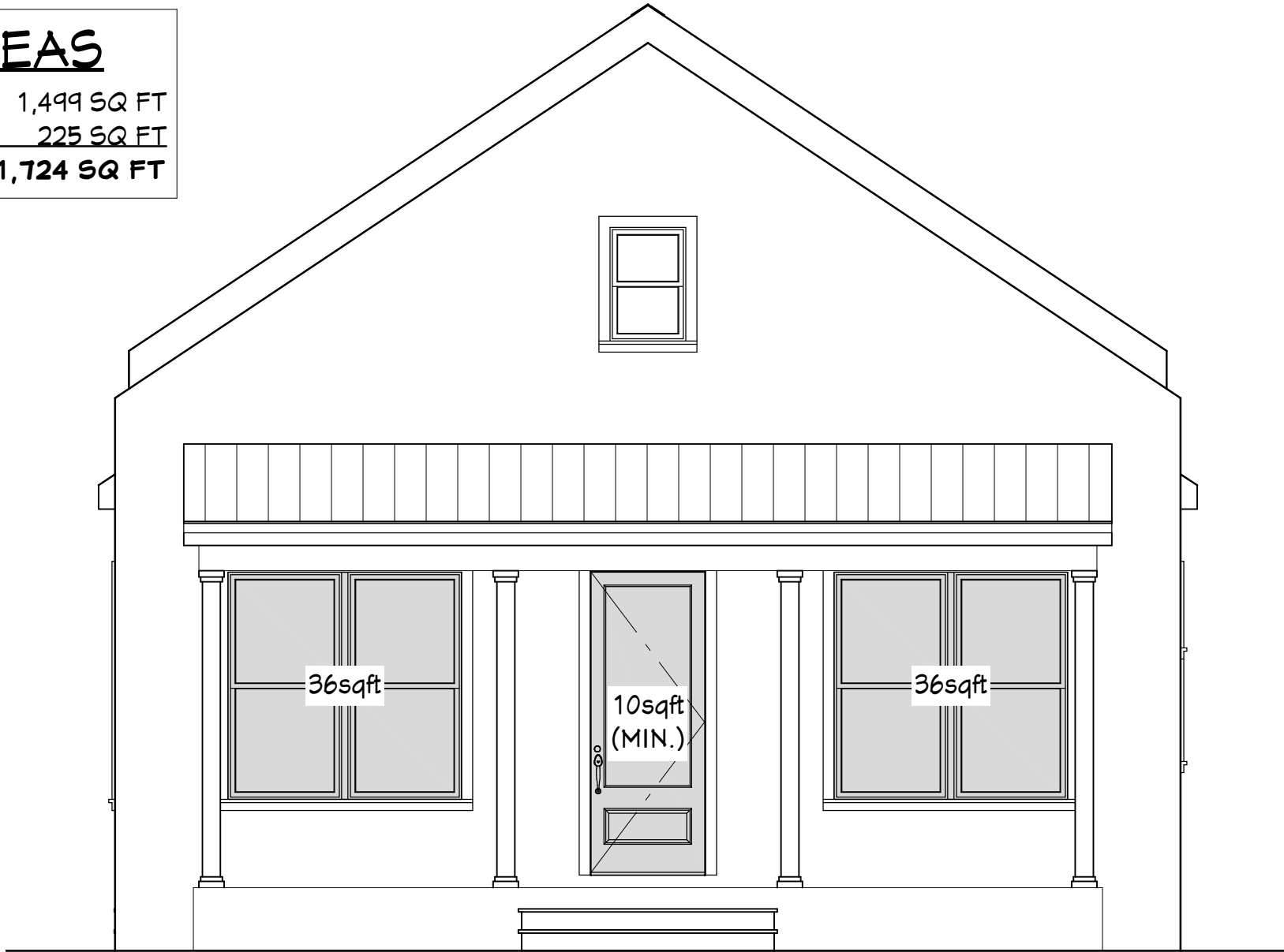
GLAZING @ FRONT ELEVATION
