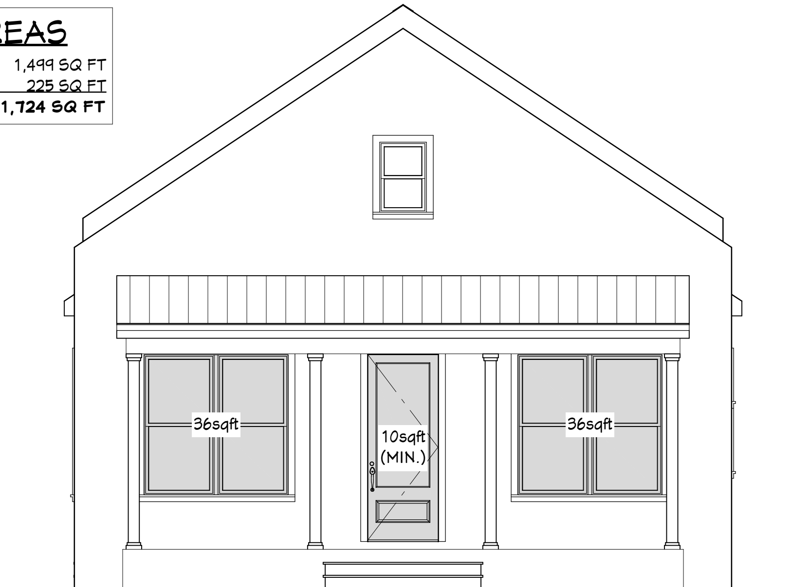
GLAZING @ FRONT ELEVATION
