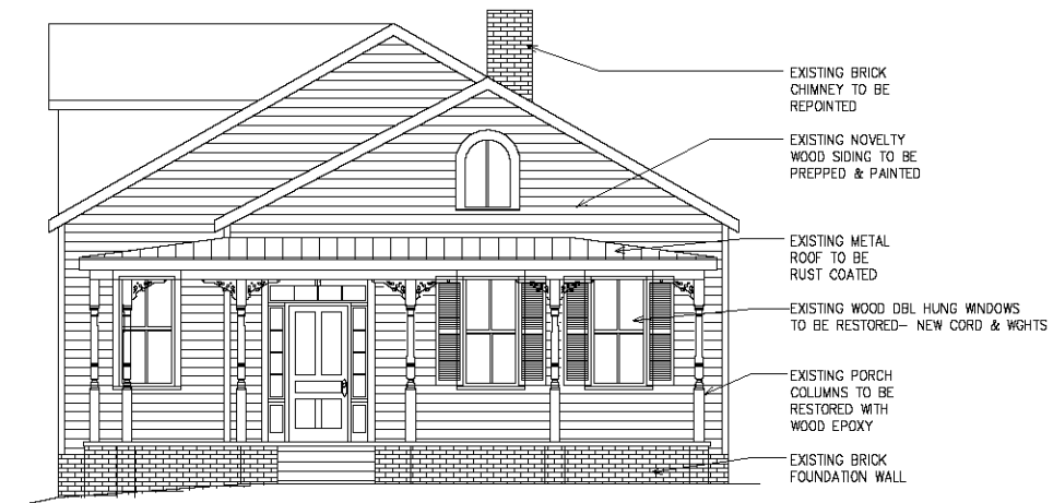
EXISTING EAST ELEVATION
