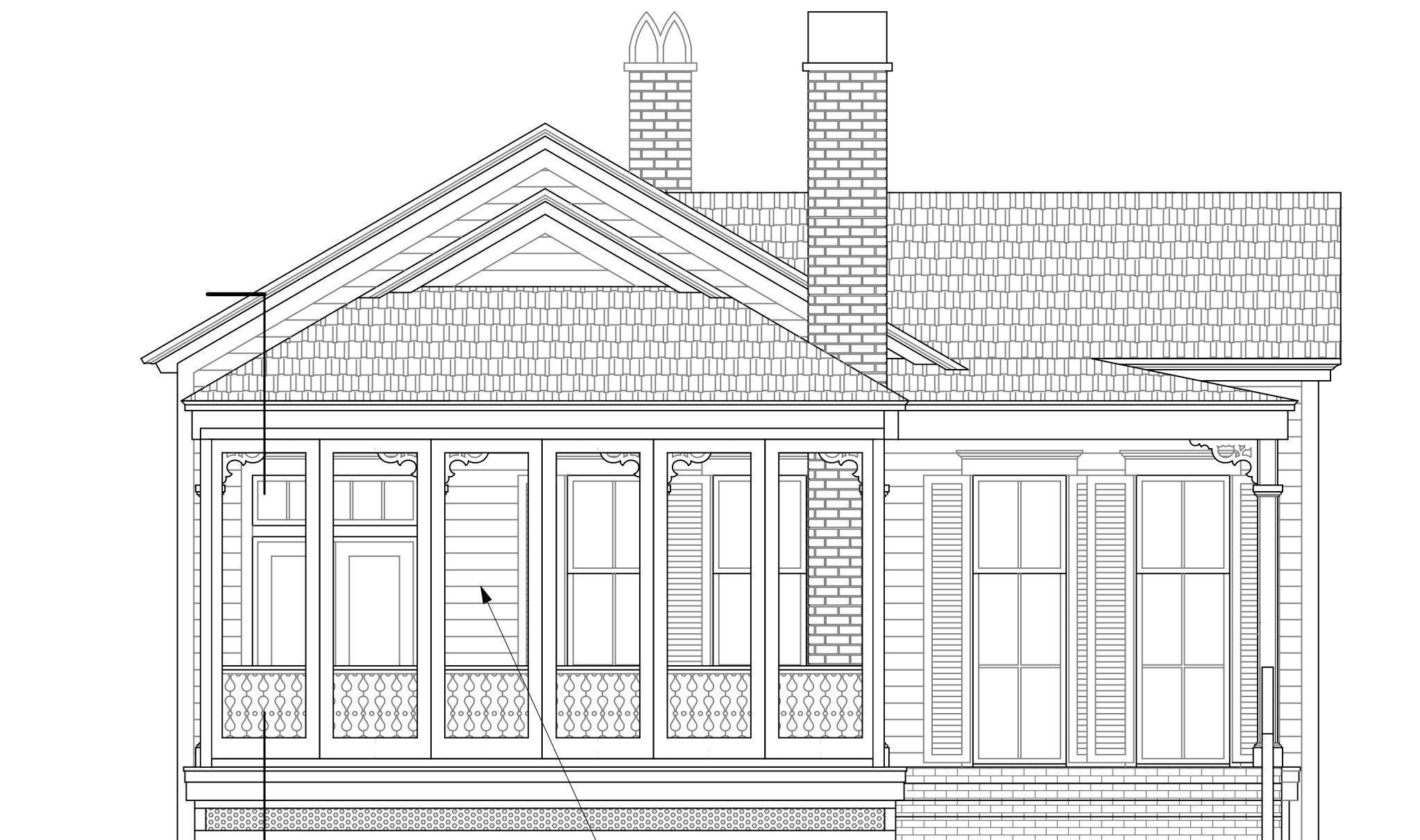
SOUTH ELEVATION SHOWING FOLDING DOOR SYSTEM WITH ALL FOLDING DOORS CLOSED
