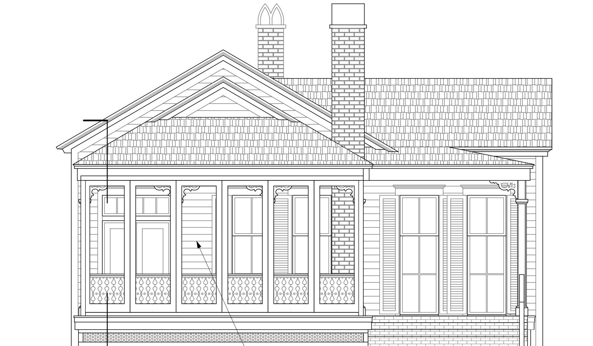
SOUTH ELEVATION SHOWING FOLDING DOOR SYSTEM WITH ALL FOLDING DOORS CLOSED
