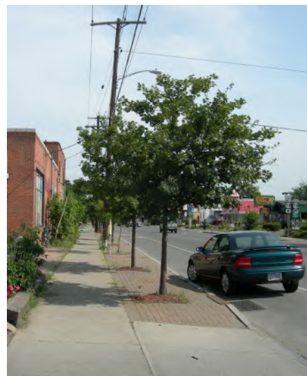
Fig. 1.24 Concrete unit pavers on a coarse sand setting bed on top of a continuous trench of CU-Structural Soil™ in Ithaca, NY
