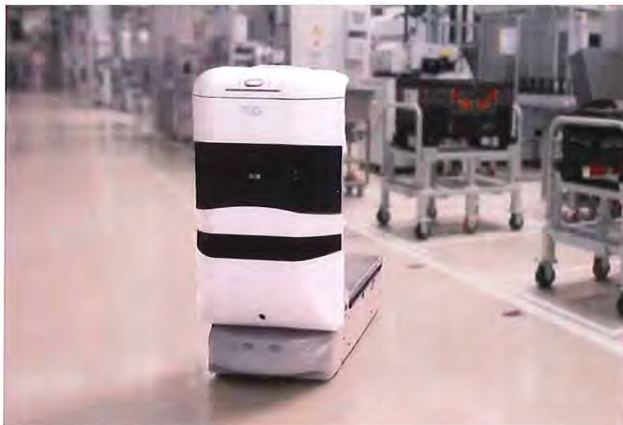
The TUG® AMR is capable of carrying loads up to 635kg.
